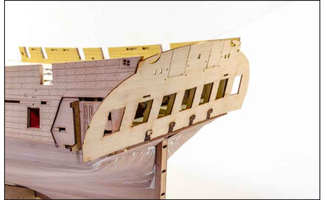
345. Slot this into the stern frames, making any adjustments as necessary for it to fully seat in the slots. DO NOT GLUE. At this stage, you can mark and paint the visible area above deck in ochre, as shown here.
