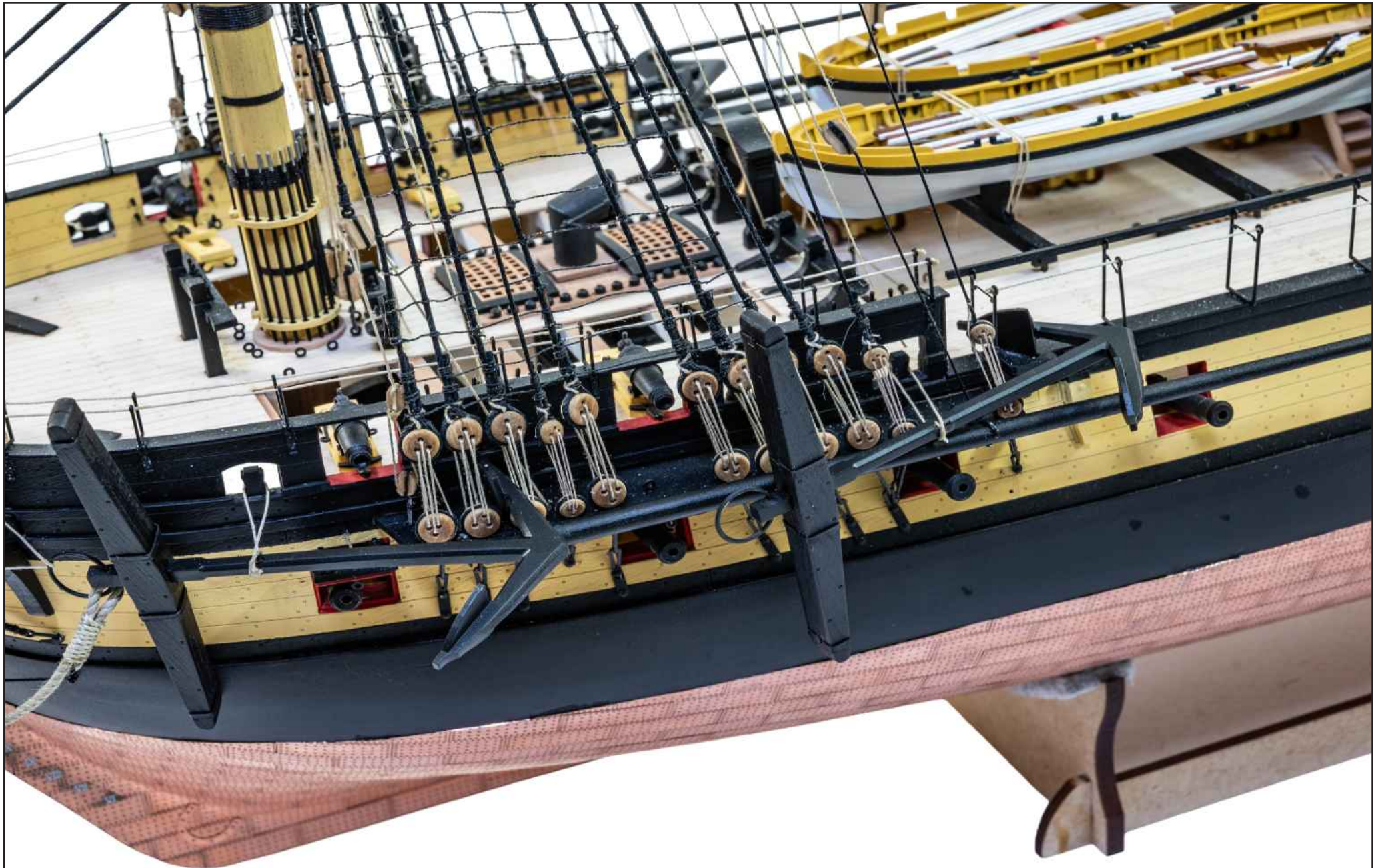
676. Hang the anchors as shown, lashing the hawse cable to them, when then slides into the hawse holes above the bolsters. Note how the rear anchor sits into the groove on the waist lower rail.
