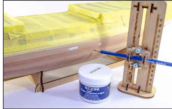
319. Checking your plans, add a temporary waterline mark BELOW the area where the final one will be. Use wood filler to fill any gaps above that line. This is the area that will be painted. The remainder of the lower hull will be coppered. We have these waterline tools in our online store.
