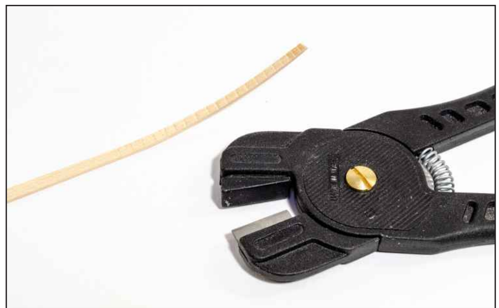
293. If necessary, you can use a plank nipping tool, or heated iron to induce a curve in the forward part of the plank.
