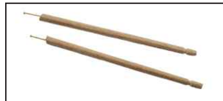
461. Referencing your plan, make the two boomkins from 3mm diameter dowel. Use brass pins (cut short) to later the boomkins to the hull.
