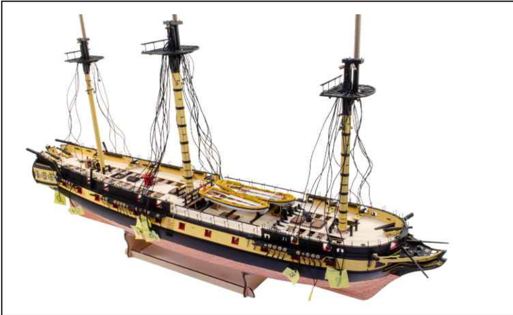
654. Using plan #16, add the lower shroud lines to each mast, taking note of sequence and diameter. The tape here is used to number the various pairs.
