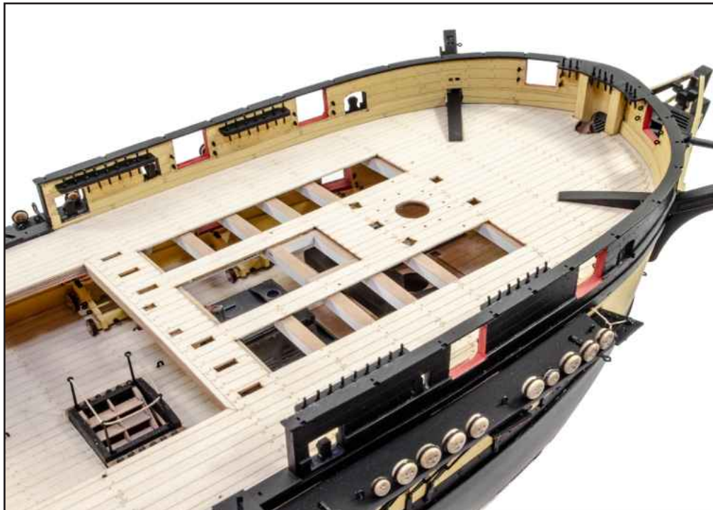
495. From the 1.5mm wood sheet, locate belaying pin racks 307 and 308. Paint black and install as shown here and on plans. From the 0.6mm PE sheet, locate belaying pins PE69. Paint black and fit to the pin racks as shown here.
