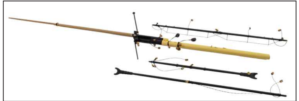
648. You can now paint and fit out the bowsprit and spritsail yard as shown. At this stage, also build and paint the Driver Gaff and Driver Boom, as shown on plan #15.
