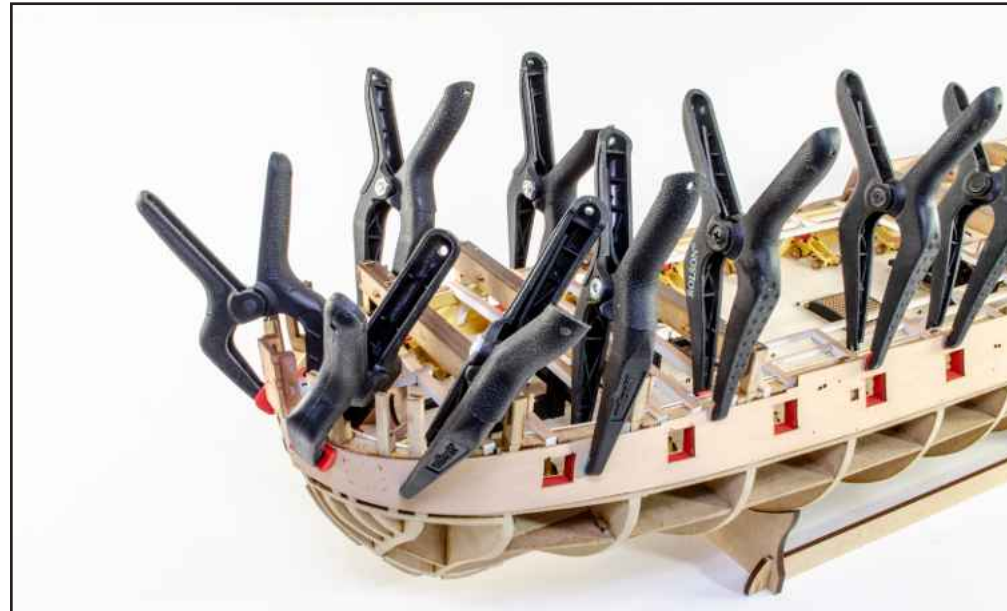
287. After drying, you can see how the ports fully align. Make sure that the part doesn't move. Do NOT glue!
