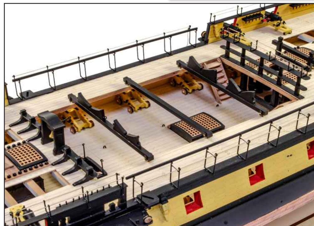
609. Use 0.5mm natural thread and rig the outer eyes of the cradles. You can also use the same rope to add a hand grab from the extra eyelet adjacent to the hull steps.
