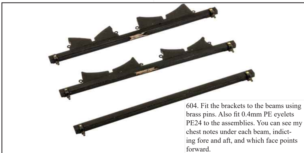
603. Using the plan measurements for reference, glue parts L3, L11, P3, and P9, from the 2mm wood sheet, onto the fore and aft beams. Paint the assemblies black. You will now need the boat beam brackets F-20.
