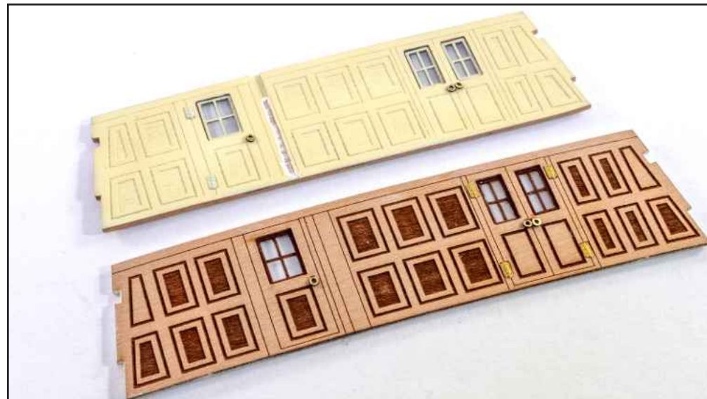
156. Glue the pairs of bulkhead screens back-to-back and allow to dry. Paint the smaller screen in an ivory colour on both sides. Use the ivory paint on only ONE side of the larger screen. That side will face towards the stern when installed. Fix the window panels into position with either odourless CA or acrylic varnish and use PE245 eyebolts from the 0.4mm PE sheet, for the door handles. You can see some paint removed on one screen here. This is where the dividing wall will be glued.
