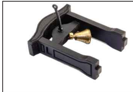
522. Paint the assembly black. Slip the brass pin through the hole in the top of the bell and bend it 90 degrees. Cut the pin to about 3mm long and then drill a hole in the underside of the assembly. Glue the bent pin into that hole so that the bell hangs within. Now glue part PE13 as shown.
