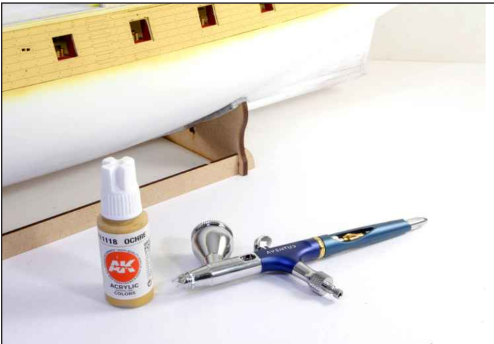
421. Now is the time to prime the hull. The reason for this is to prepare the hull and identify any defects in the woodwork, that would ruin the overall look of your completed work. We recommend both Tamiya Fine White primer or Plastikote White primer. With this on, fill and rub back any defects and lightly re-prime. The first colour to be applied is Ochre. We recommend the AK paint available in our store.
