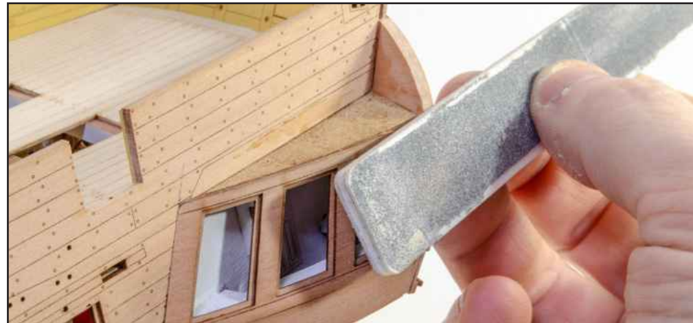
368. Sand the edges of the laminated stern construction as shown, ensuring it is smooth along its length.
