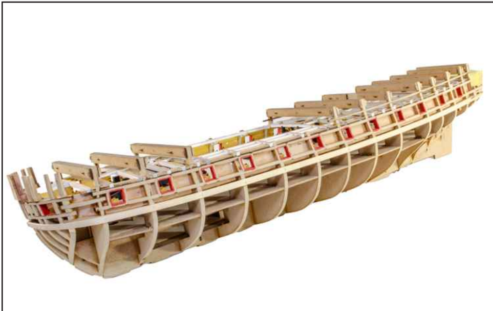
290. Here is an overall view of the first fitted plank. From here, you will need to taper the planks, so they conform properly to the hull.
