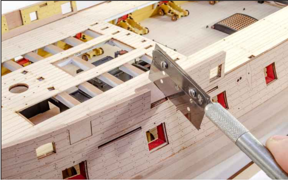
330. Carefully remove the various port/opening blanks in the forecastle bulwarks. A good quality razor saw is perfect for this.
