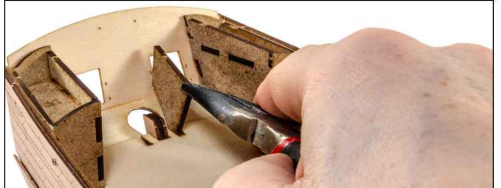
138. Install part 166 as shown here. Ideally, you need to paint these parts before assembly. For our prototype, we created an ivory colour by mixing matt white with a touch of ochre paint.
