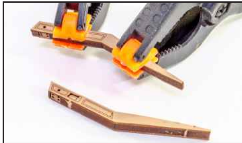
335. Now glue the appropriate side panels onto the 2mm parts and clamp until dry.
