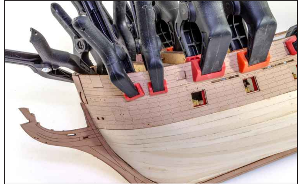
315. Now glue and clamp the parts into place as shown and leave to thoroughly dry. Make sure the various opening sections are aligned.
