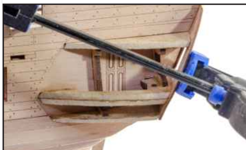
354. The stern inner panel can now be glued into place and then clamped up to the quarter gallery MDF frames until the glue is set.
