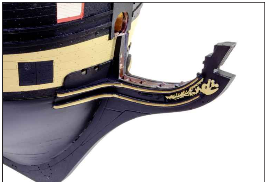
423. Paint the bow areas in ochre as shown and paint/glue parts 283 and 284, from the 0.6mm PolyBak sheet, as shown.
