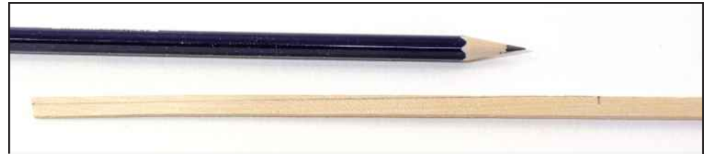
291. To taper a plank, gently bend around the bow and make a mark where it begins to cross over the previous plank. Now make a mark about 1/3 down the width of the plank, at the front. Draw a line to connect the marks.
