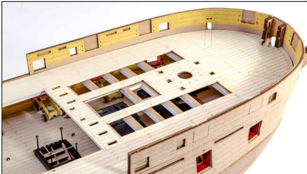
326. Once dry, paint the upper section of these parts in ochre and then glue/clamp into place until dry.
