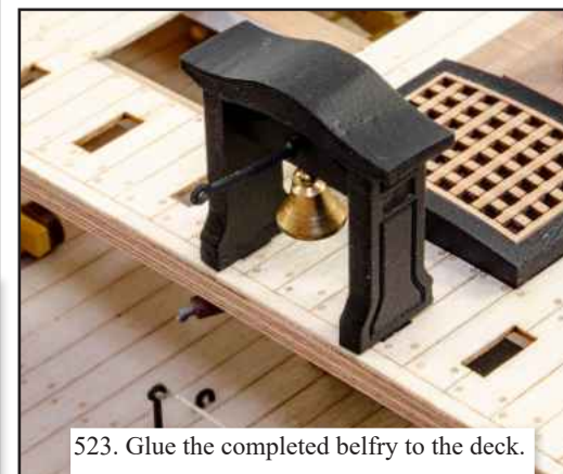
522. Paint the assembly black. Slip the brass pin through the hole in the top of the bell and bend it 90 degrees. Cut the pin to about 3mm long and then drill a hole in the underside of the assembly. Glue the bent pin into that hole so that the bell hangs within. Now glue part PE13 as shown.
