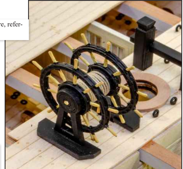
568. Glue the unit into position, threading the ends of the cord through the holes in the deck.
