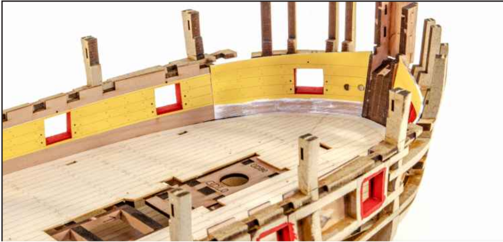
146. Install the same opposite parts within the opposite hull side and then finally install the previously soaked inner bow parts, after painting in ochre.
