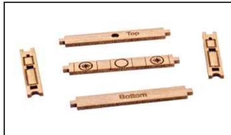
569. LARGE BINNACLE: For Surprise, we provide TWO binnacles, so you can choose your own and its location. Here we see the larger one being built. From the 1mm sheet, remove parts OB3, OB4, OB5, and OB6.
