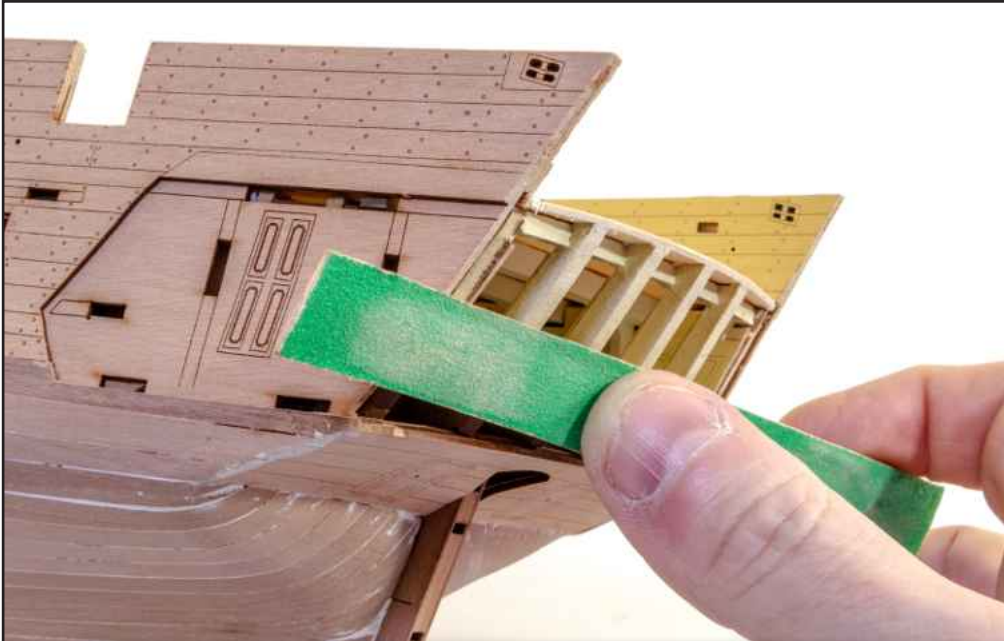
343. Now we look at the stern of Surprise. Use a sanding stick to flush any protrusions at the rear end, including levelling off the bulwarks and deck so they flow with the curves of the stern frame timbers. Be careful not to sand away the protruding slots in the stern frame timbers.
